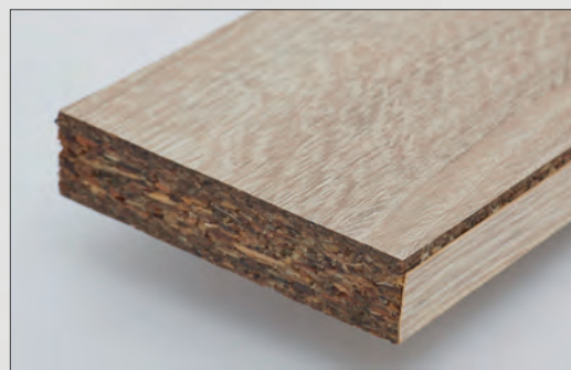
Above: non-water-repellent chipboard before, and after, soaking in water for 24 hours
